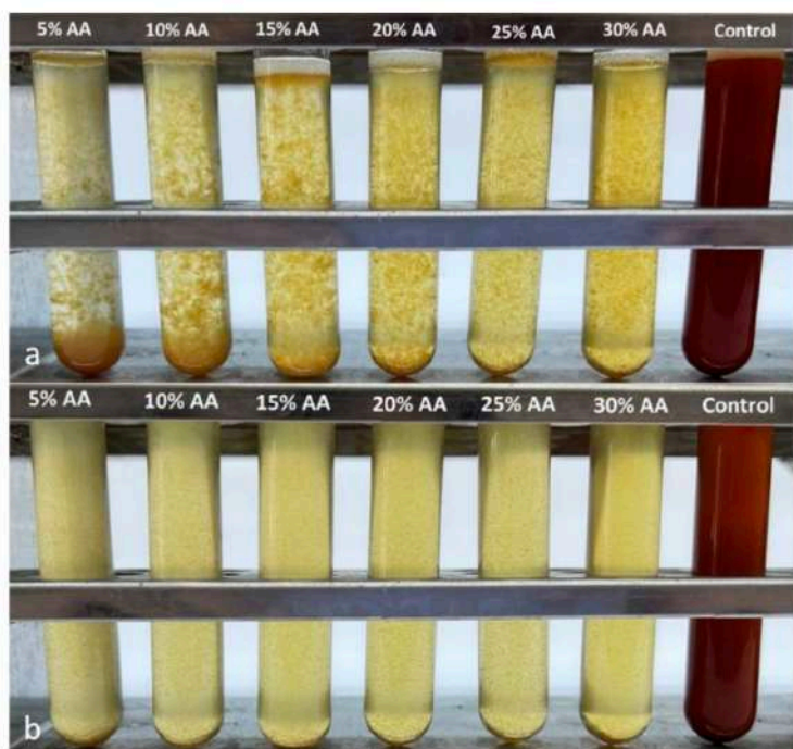
Figure 2. Photographs of test tubes to which 5 mL of AA (a) and 10 mL of AA (b) were added at specific concentrations.
