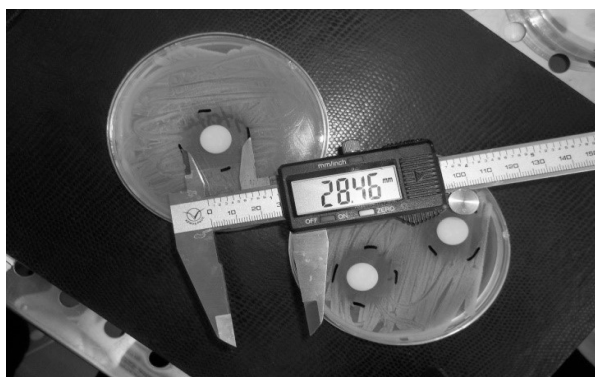
Figure 1. Measuring the inhibition zone with a digital caliper
